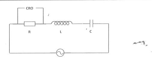
When an input signal  $V_{in} = V_o e^{i\omega t}$  is given to the circuit above, the current through the above circuit is given by  $I = \frac{V_o}{\sqrt{R^2 + \left(\omega L - \frac{1}{\omega C}\right)^2}} e^{j(\omega t - \phi)} = I_o e^{j(\omega t - \phi)},$
