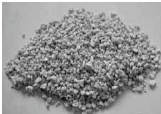
**Figure 3.22:** Pumice aggregate (under 4mm sieve)
